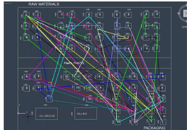
Figure 1 Material flow of existing layout
