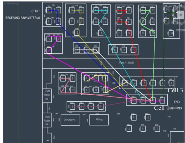
Figure 4 Proposed layout (rectangle shapes around several machines represent layout modules and numeric values inside square shapes represent the machine types)
