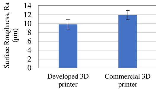
Figure 5: Surface roughness comparison between in-house developed 3D printer and commercial 3D printer
