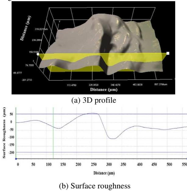
Figure 3: Surface profile of part fabricated using open source 3D printer
