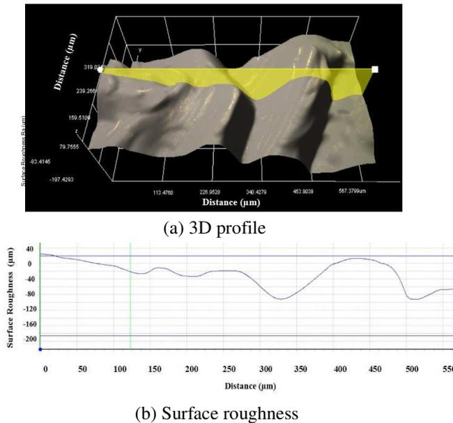
Figure 4: Surface profile of part fabricated using commercial 3D printer
