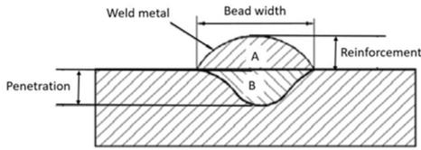
Figure 1 Weld bead geometry characteristics[2]
