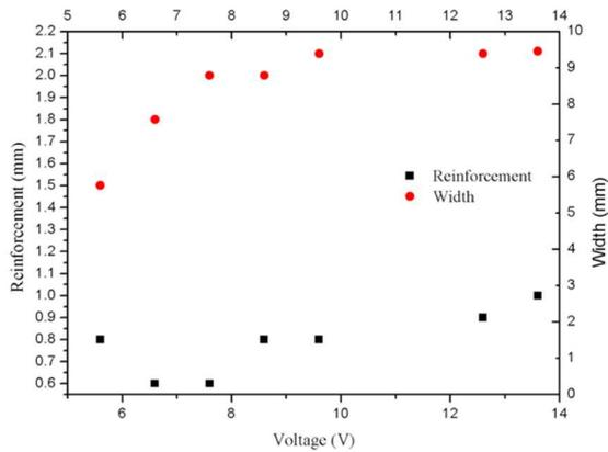
Figure 2 The effect of welding voltage on reinforcement and bead width
