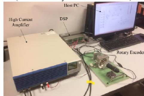
Figure 1 SRA experimental setup for measuring the rotary motion characteristics
