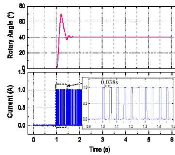
(b) Pulse signal 20Hz, 1:4 duty ratio
