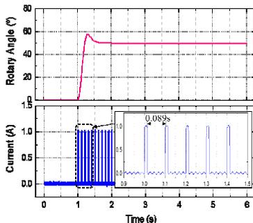
(a) Pulse signal 10Hz, 1:4 ratio
