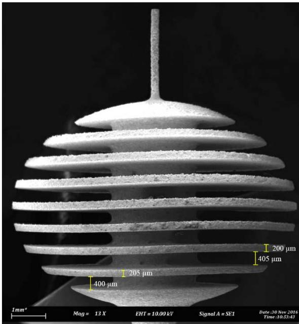
Figure 2 SEM of fabricated micro fins features by slitting operation on ellipse shapes
