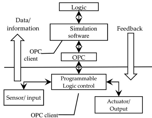
Figure 1: Base structure for automation CPS for material handling system equipment
