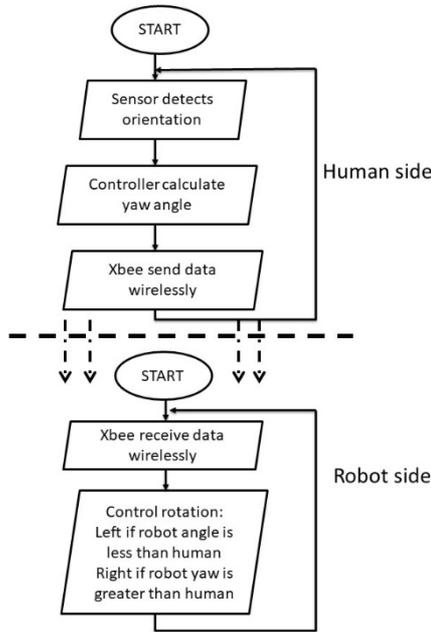
Figure 2. Flowchart of the yaw tracking system
