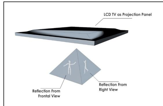
Figure 5 i-HO Projection Panel Setup
