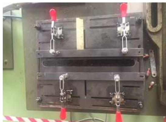
Figure 2 Jig for thin plate welding
