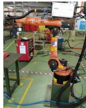
Figure 1 The Robotic Arm of Gas Metal Arc Welding KRC4 Type (GMAW) (FKP Welding Laboratory)
