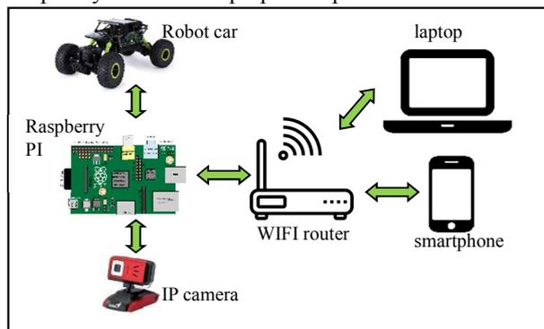
Figure 1 Prototype Concept Diagram
