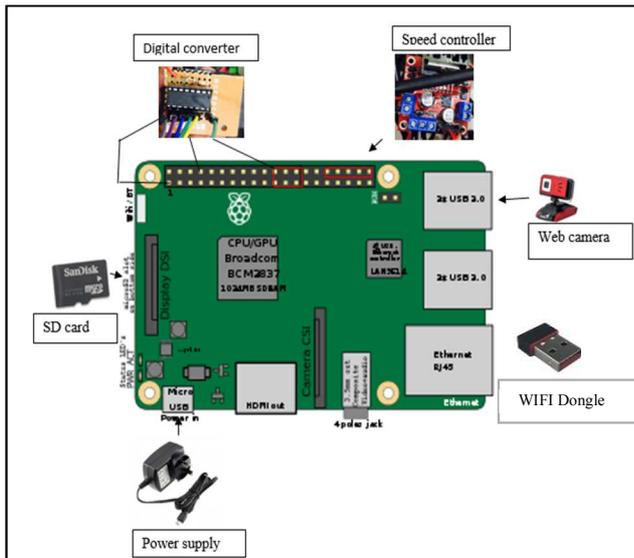
Figure 2 Physical Design of Raspberry Pi Robot Car Board Controller with pin configuration
