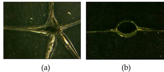
Figure 3: Cracked pattern under lower (a) and higher (b) thrust force
