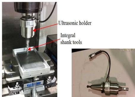
Figure 1: Rotary ultrasonic drilling setup and tool holder
