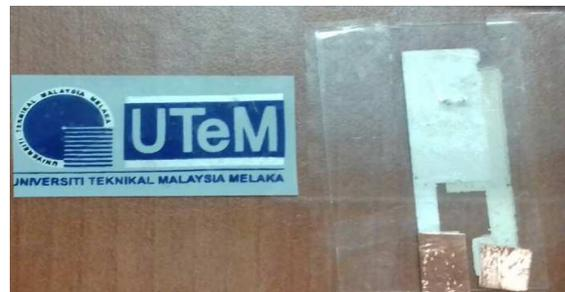
Figure 2 Fabricated P(VDF-TrFE) thick film
