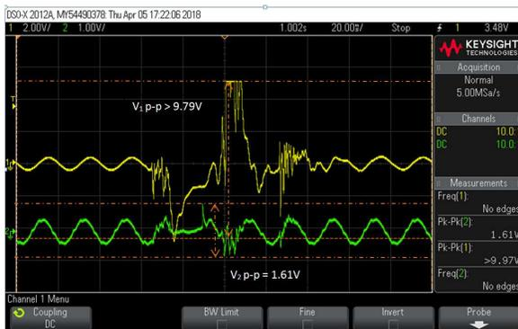
Figure 5 Output voltage using different blocks for hot plate polling
