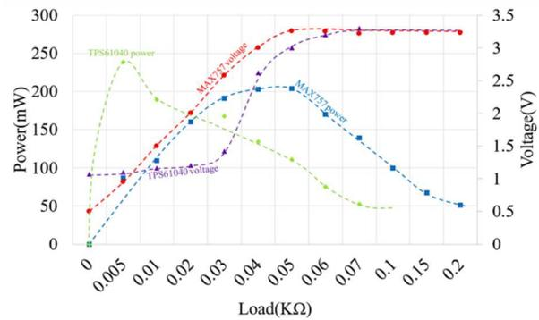
Figure 4: Power and voltage of both MAX and TPS.
