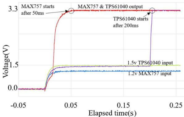
Figure 3: The starting points of both MAX and TPS.
