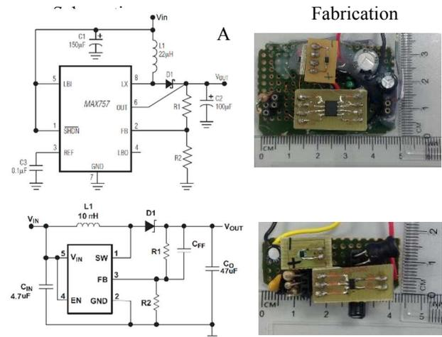
Figure 1: The schematics and the fabricated circuits for A-MAX757, B-TPS61040.
