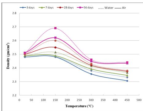
Figure (2): The Density of RPC samples at different Fire Flame.
