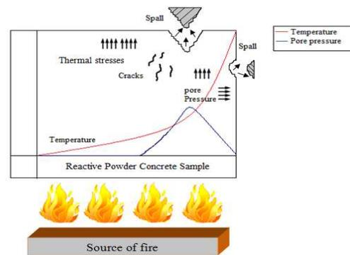
Plate (1): expected mechanism of Spalling behavior of RPC Samples affected by Real Fire Flame.
