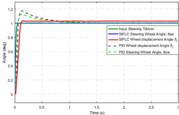
Figure 3 Step response for  $\theta_{sw}$  and  $\delta_f$  for SIFLC and PID-PID
