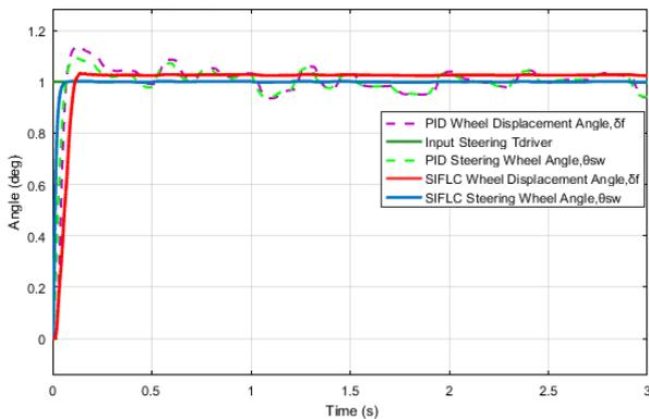
Figure 4 Step response for  $\theta_{sw}$  and  $\delta_f$  for SIFLC and PID-PID with disturbance.
