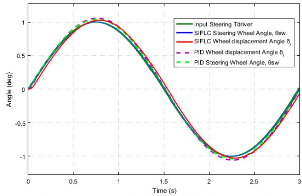
Figure 5 Sinusoidal response for  $\theta_{sw}$  and  $\delta_f$  for SIFLC and PID-PID.
