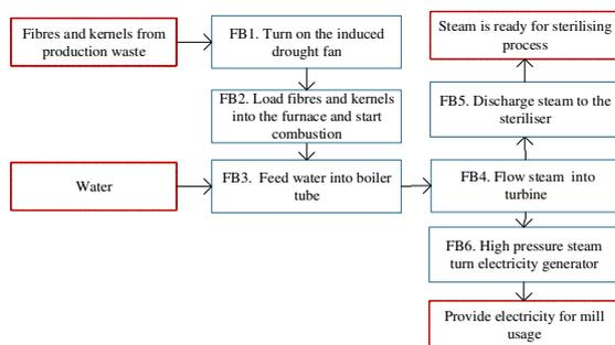
Figure 3: Functional Block Diagram of Boiler
