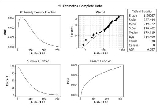
Figure 2: PDF, Goodness-Of-Fit, Survival, and Hazard Rate Plot of Boiler
