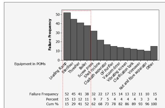
Figure 1: Frequency of Equipment Failure in the POM
