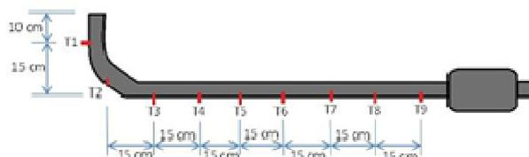
Figure 1 Schematic of thermocouples location along the exhaust pipe
