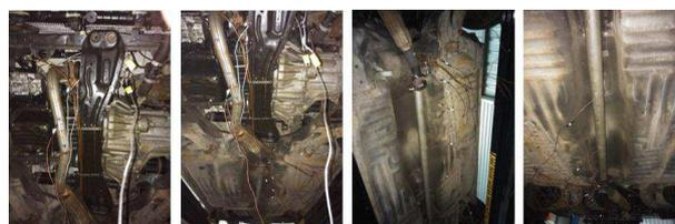
Figure 2 Thermocouple point location on the experimental vehicle
