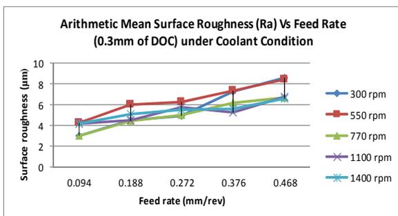
Figure 2 Arithmetic mean surface roughness (Ra) Vs feed rate under coolant condition
