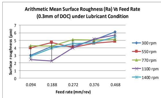
Figure 3 Arithmetic mean surface roughness (Ra) Vs feed rate under lubricant condition
