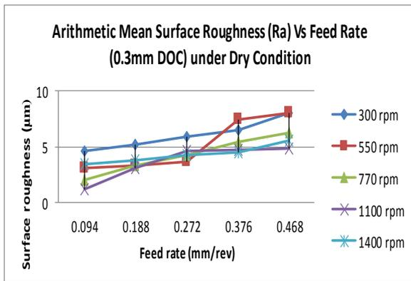
Figure 1 Arithmetic mean surface roughness (Ra) Vs feed rate under dry condition
