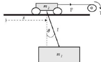
Figure 1 Schematic diagram of a gantry crane [1]
