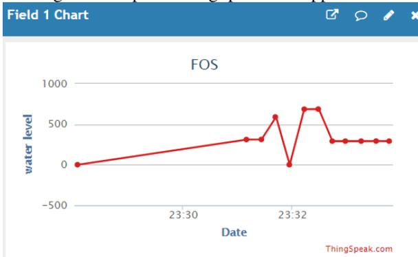
The results shown in both Figure 1 and 2 are obtained from the sensor unit. The changes in the graph indicate the changes in the water level and it is plotted in real-time. Both data can be exported and used for offline research. When the water level increases, the distance between water and sensor will decrease, this will indicate that the water level is increasing. When this happens, the water level in the graph will increase.
