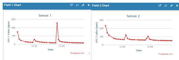
Figure 3: Thingspeak IoT data showing two sensors separated by 2 meters apart and source of LPG were tested from different places.
