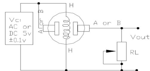
Figure 1: LPG sensor circuit.
