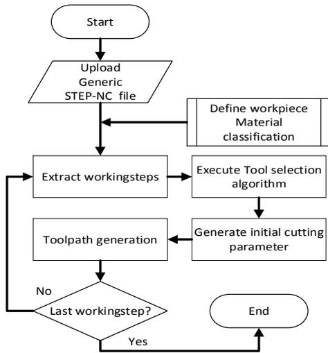
Figure 2. The process flow of native CNC planning
