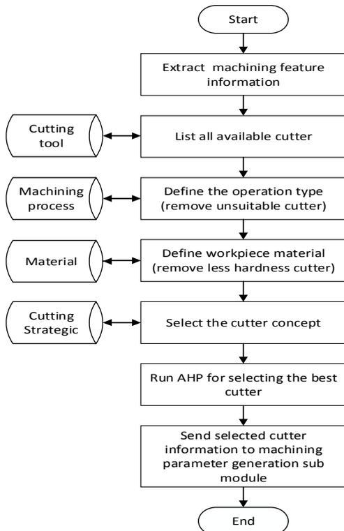
Figure 3. Cutting tool selection procedure
