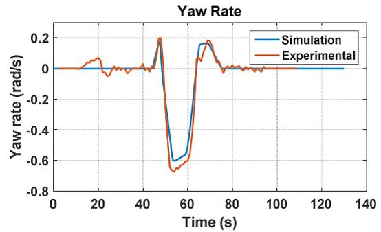
Figure 4 Comparison of yaw rate of experimental and simulated result.
