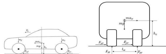
Figure 2 (a) Mass distribution and forces acting on vehicle, (b) Load transfer on vehicle [3]
