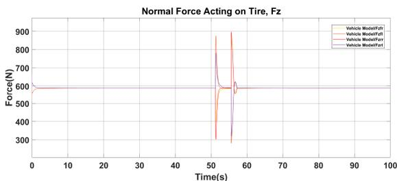
Figure 5 Normal force,  $F_z$  acting on tire
