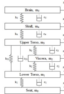
Figure 1 Schematic of 5DOF model [4-5]
