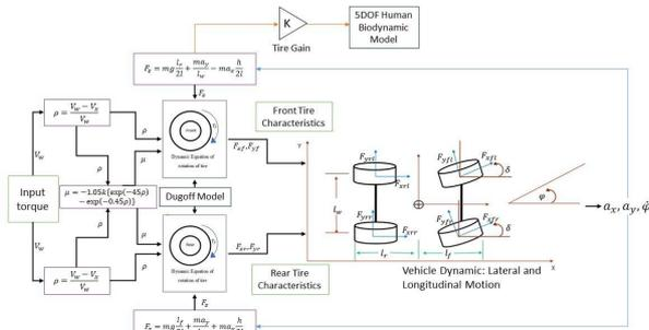
Figure 3 Schematic diagram of vehicle and human biodynamic model
