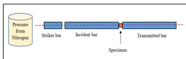
Figure 1 Schematic of SHPB
