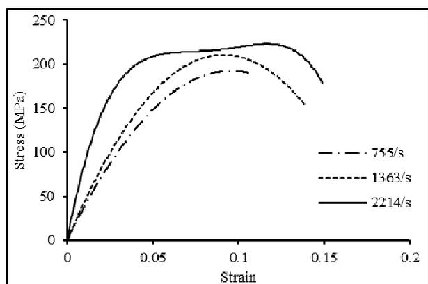
Figure 2 Stress-strain curves of E-glass/jute
