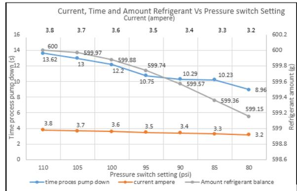
Figure 3: Recovered refrigerant amount, time taken and current supply for different pressure setting
