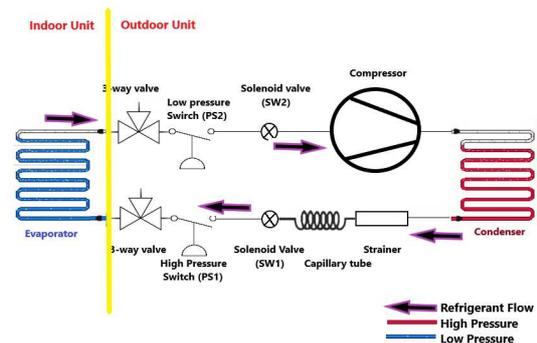
Figure 1: Installation of additional switch and valves
