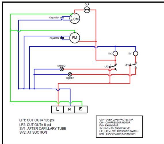
Figure 2: Diagram of wiring modification on experimental unit
