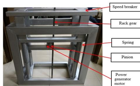
Figure 1 Prototype of road power generator
