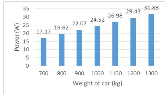
Figure 5 Vehicles weight vs power generated for 15 cm speed breaker height
