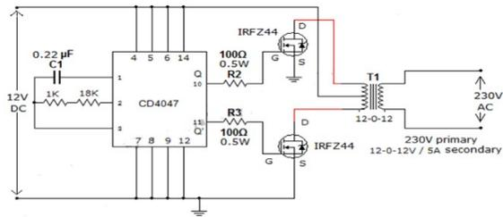
Figure 3 Inverter circuit
