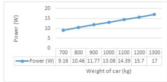
Figure 4 Vehicles weight vs power generated for 8 cm speed breaker height
