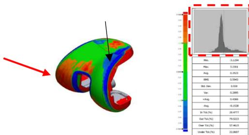
Figure 4 Result of dimensional accuracy analysis – Multi-Axis Sweeping
