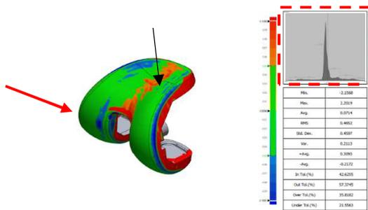
Figure 3 Result of dimensional accuracy analysis – Isoparametric
