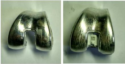
Figure 2 Machined femoral knee – Isoparametric (left) Multi-Axis Sweeping (right)
