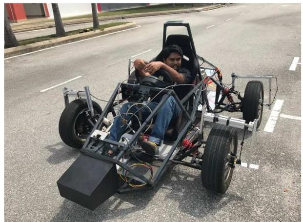
Figure 1 The two in-wheel vehicle prototype with sensors used in the research to obtain the vehicle parameters.
