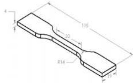
Figure 1 Test specimens, all dimensions are in mm: tensile test specimen
