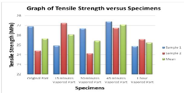
Figure 3 Graph of tensile strength versus specimens
