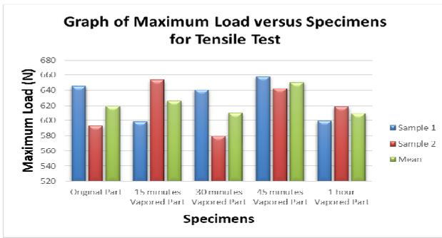
Figure 2 Graph of maximum load versus specimens for tensile test
