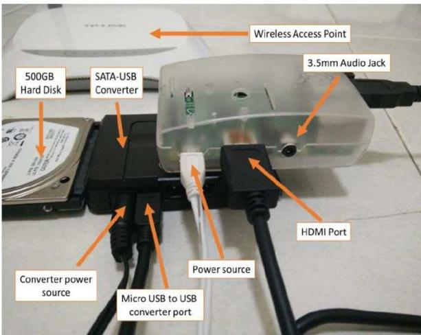
Figure 2 Portable Wireless Cloud Storage hardware
