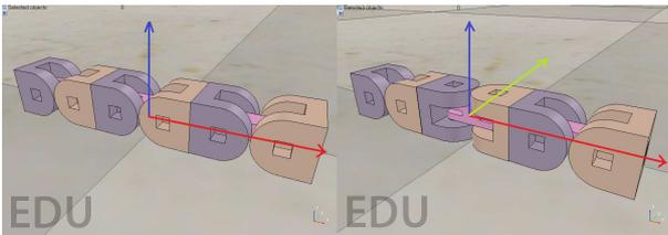
Figure 2 Uniform attachment position (Left) and irregular attachment position of robot (Right)
