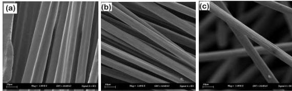
Figure 1 SEM images (500X magnification) of recycled carbon fiber in CFRP after different treatments: (a) untreated; (b) chemically treated and (c) chemically and mechanically treated into size of about 90  $\mu\text{m}$ .
