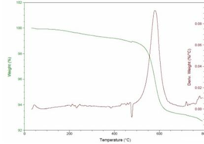
Figure 3 TGA curves of chemically treated rCF
