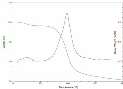
Figure 2 TGA curves of untreated rCF
