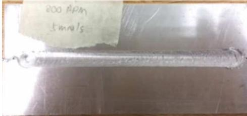
Mitra *et al* [4] reports the main effect is a value which shows the extent influence of a factor on the response. Hence, the combination for optimum parameter condition is A1B1 (800 RPM, 5mm/s) that will give the optimum tensile test.
