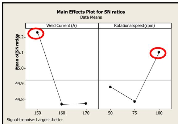
Figure 3 Main effects plot for S/N ratios of microhardness response
