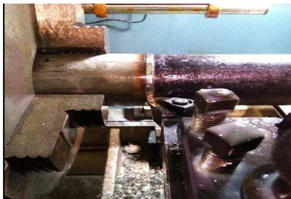
Figure 2 Grinding using lathe machine
