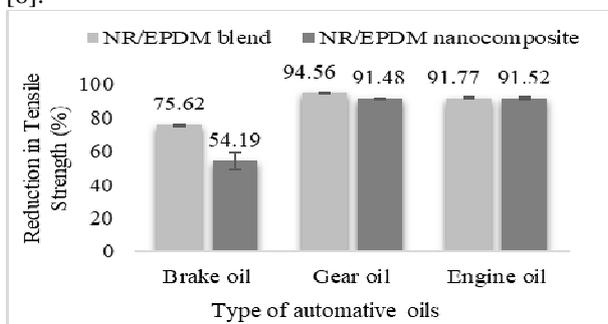
Figure 1 Reduction of tensile strength in different types of automotive oils.
