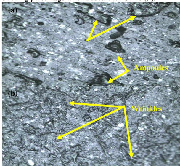
Figure 2 OM of (a) NR/EPDM blend in gear oil, and (b) NR/EPDM nanocomposite in gear oil at 200x mag.
