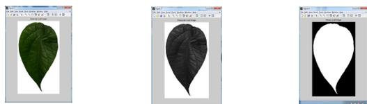
a. Load Image b. RGB- grayscale c. Otsu method
