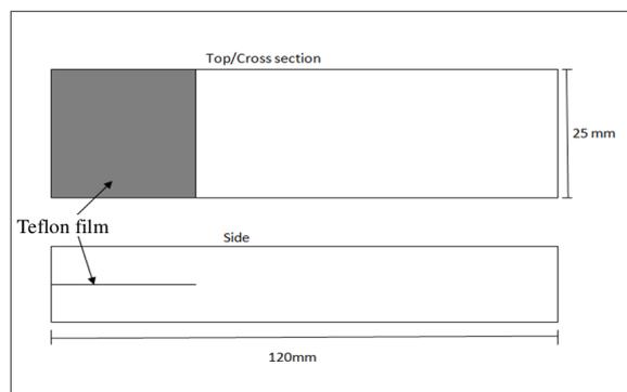
Figure 1 Schematic orientation of coir fiber and Teflon film
