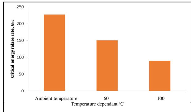
Figure 2 Graph of critical energy release rate,  $G_{IIC}$  for each composite sample of coir fiber
