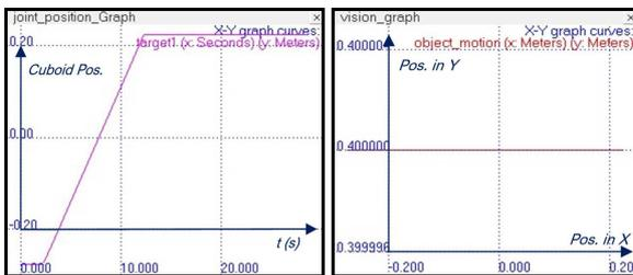
Figure 5 Graphs of (a) movement pattern for youBot joint and (b) position for youBot joint in part A
