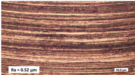
Figure 2 Optical microscopic image of milled surface roughness at 0 kHz
