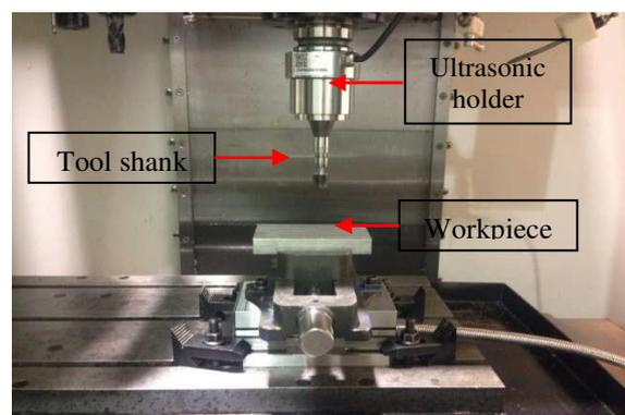
Figure 1 The setup of the ultrasonic vibration on the CNC Milling
