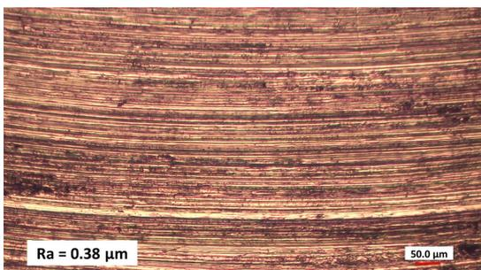
Figure 3 Optical microscopic image of milled surface roughness at 27 kHz
