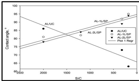
Figure 1 Contact angle at different SiC roughness
