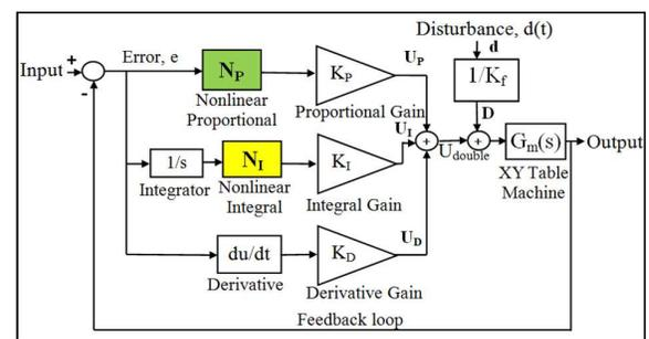
Figure 1: NPID Double Hyperbolic Controller Scheme
