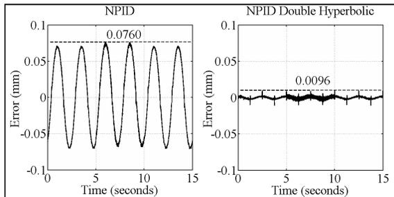
Figure 3: Experimental Result for Speed of 0.4 Hz
