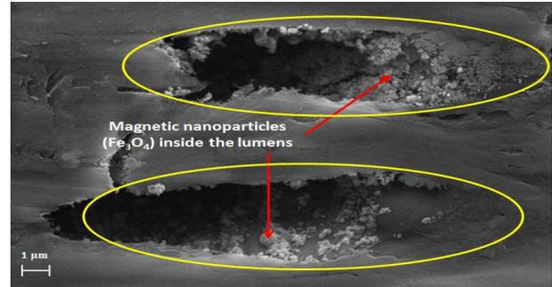
Figure 3 SEM micrograph of magnetite nanoparticles inside the durian shell lumens fibre of the nanocomposite sheet
