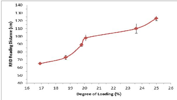
Figure 1 Graph of RFID reading distance in metallic environment versus degree of loading of magnetite
