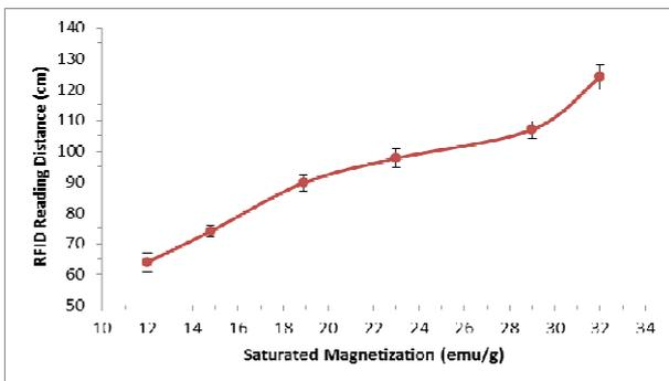
Figure 2 Graph of RFID reading distance in metallic environment versus saturated magnetization
