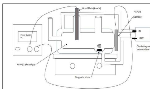
Figure 1 Schematic diagrams of electrodeposition process
