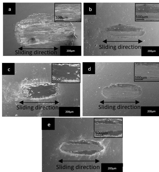
Figure 5 SEM image of wear scar:a) Bare AA7075, b) Pure nickel, c) Ni-P, d) Ni-P-QD 50 g/l, e) Ni-P-QD 50 g/l (400°C)
