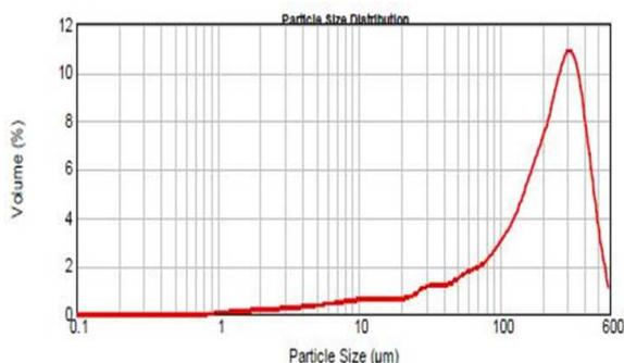
Figure 2 Particle size distribution of quarry dust
