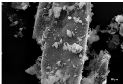
Figure 3 SEM image of quarry dust particles
