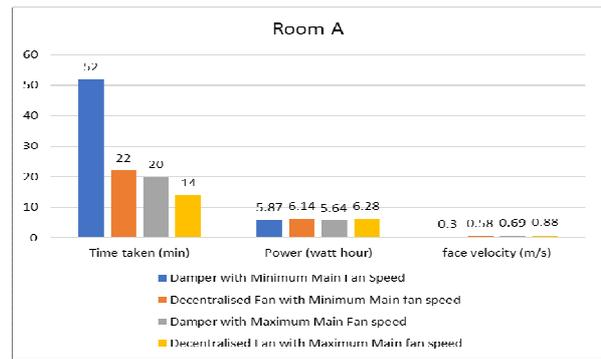
Figure 5 Time taken to cool, power consumption and face velocity for room A
