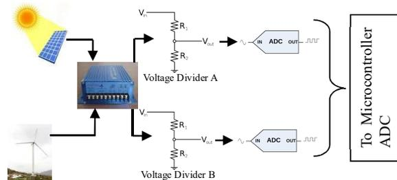
Figure 1 Solar – Wind hierarchical voltage sensing – voltage divider method
