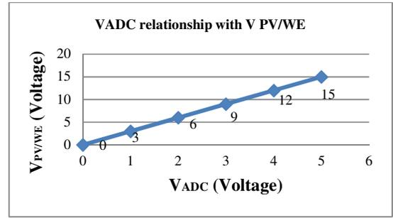
Figure 2  $V_{ADC}$  proportion relationship with  $V_{PV/WE}$
