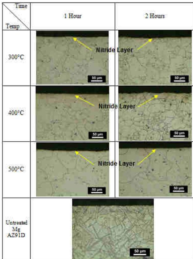
**Figure 2** Optical microscopic images of cross section of the untreated and the nitrided MgAZ91D with regard to temperatures and nitriding time.
