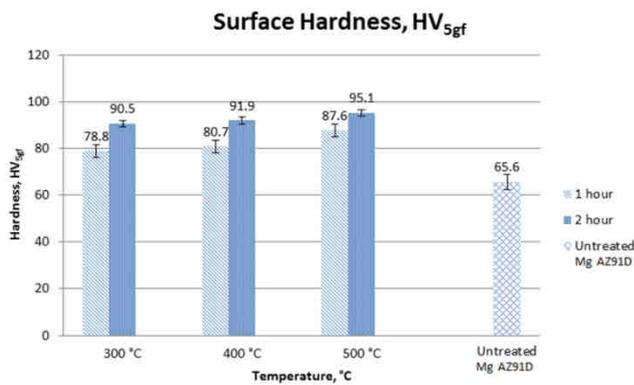
**Figure 1** Surface hardness of the untreated MgAZ91D and nitrided MgAZ91D with different temperatures and nitriding time.
